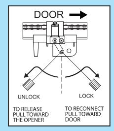
FIG. 6-3 Engage/Disengage Carriage Lock.
